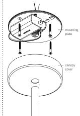
The client is responsible to ensure fasteners are attached to a robust structural substrate.
